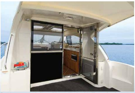
From the stern we see the large stainless steel hatch and the lift up awning window.
