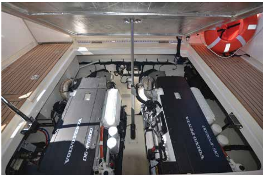
The large engine room hatch opens hydraulically at the touch of a switch to provide excellent access to the engine room for checks and service.
