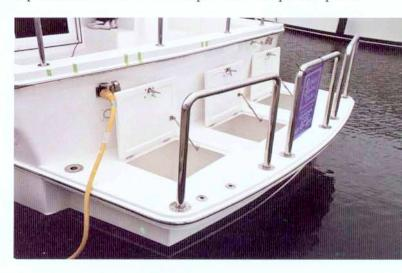
water to drain to the lowest point allowing the sump pump to expel the water. The sport box has a multitude of uses, including miscellaneous gear storage, dive gear, bladder bags for extra fuel capacity and for the fisherman, a fish box.
